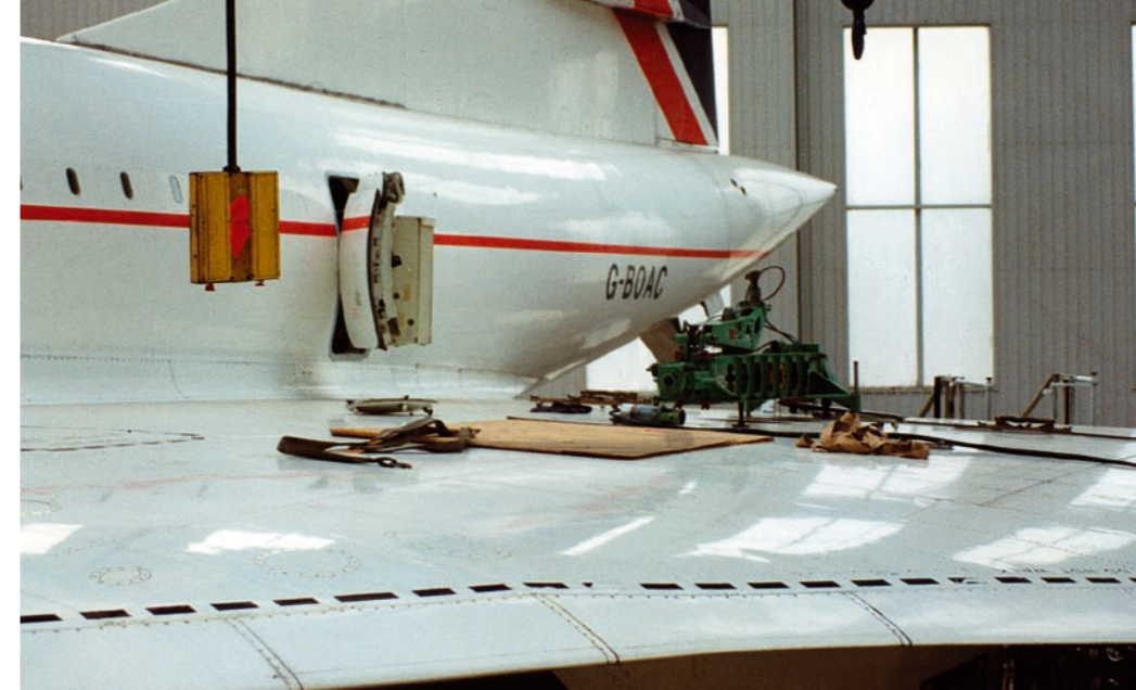
LEFT A Sabena hoist in position on top of the wing, ready for an engine change. David Macdonald
