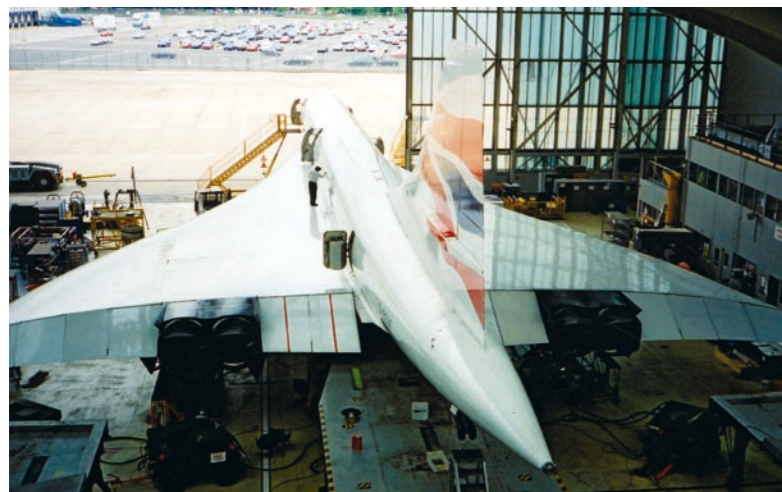
ABOVE AND ABOVE RIGHT The Minor Maintenance Team looks after the Service Check, scheduled every 175 flying hours. John Dunlevy/Carl Percey
